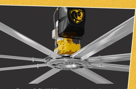
Powerfoil X4®'s gearbox is hermetical sealed, and its VFD is housed in a custo ABS enclosure with a built-in heatsink operate at peak performance in even that harshest conditions. Its c-face motor make servicing a breeze—motor replacement possible in as little as an hour.
